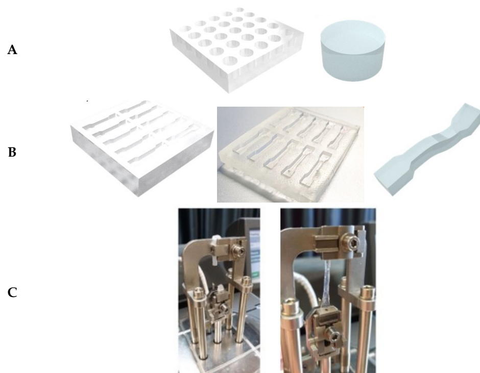
Figure 15. Samples used for the DMA analysis. (A) Circular samples for compression tests. (B) Dog-bone samples for tensile tests. (C) Real photos of the hydrogel dog-bone samples under tensile stretching.
