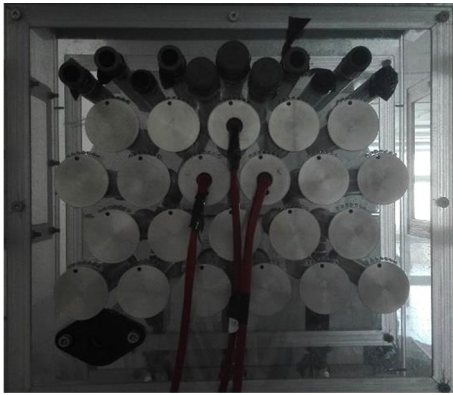
Fig. 2 Staggered tubes setup. Rotating elliptical tubes, the right inclination can be reached (reference pin holes were drilled ad hoc in the transparent wall of the test section)
