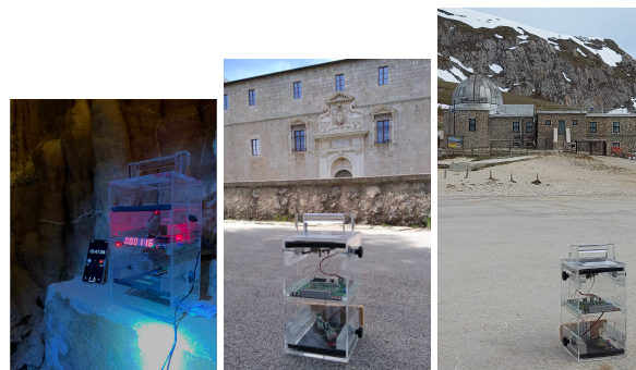
Figure 2: Cosmic Box used to study muon rate at different altitude. From left to right: -20 m under ground level, 750 m and 2112 m above sea level.
