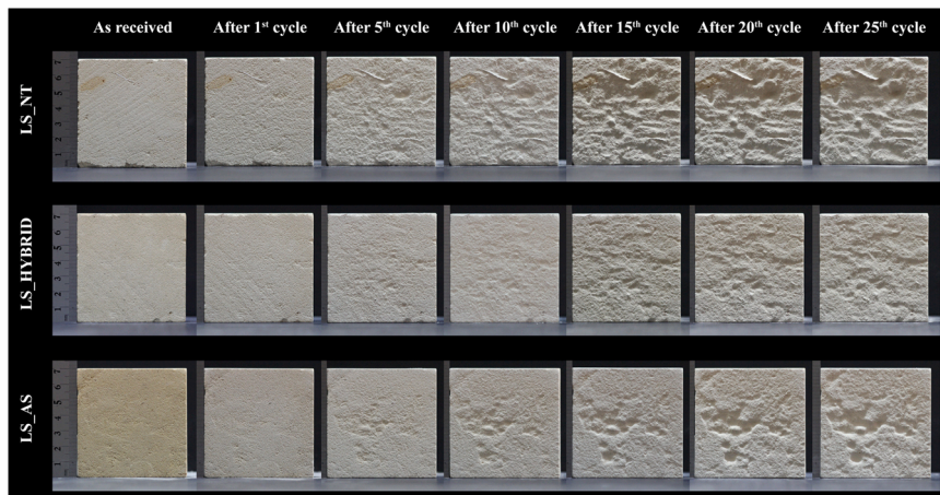
Fig. 3. LS_NT, LS_HYBRID and LS_AS samples during erosion test.
