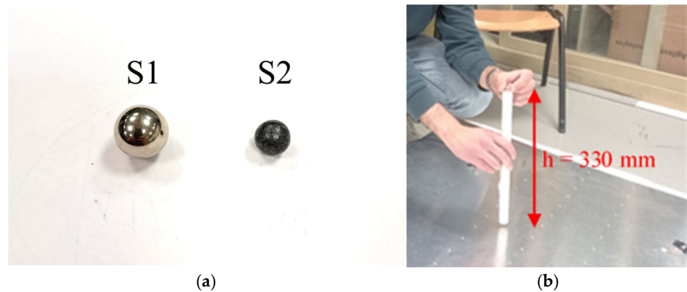
Figure 3. The spheres used for generating the impact on the plate surface (a) and a detailed image of the process (b).
