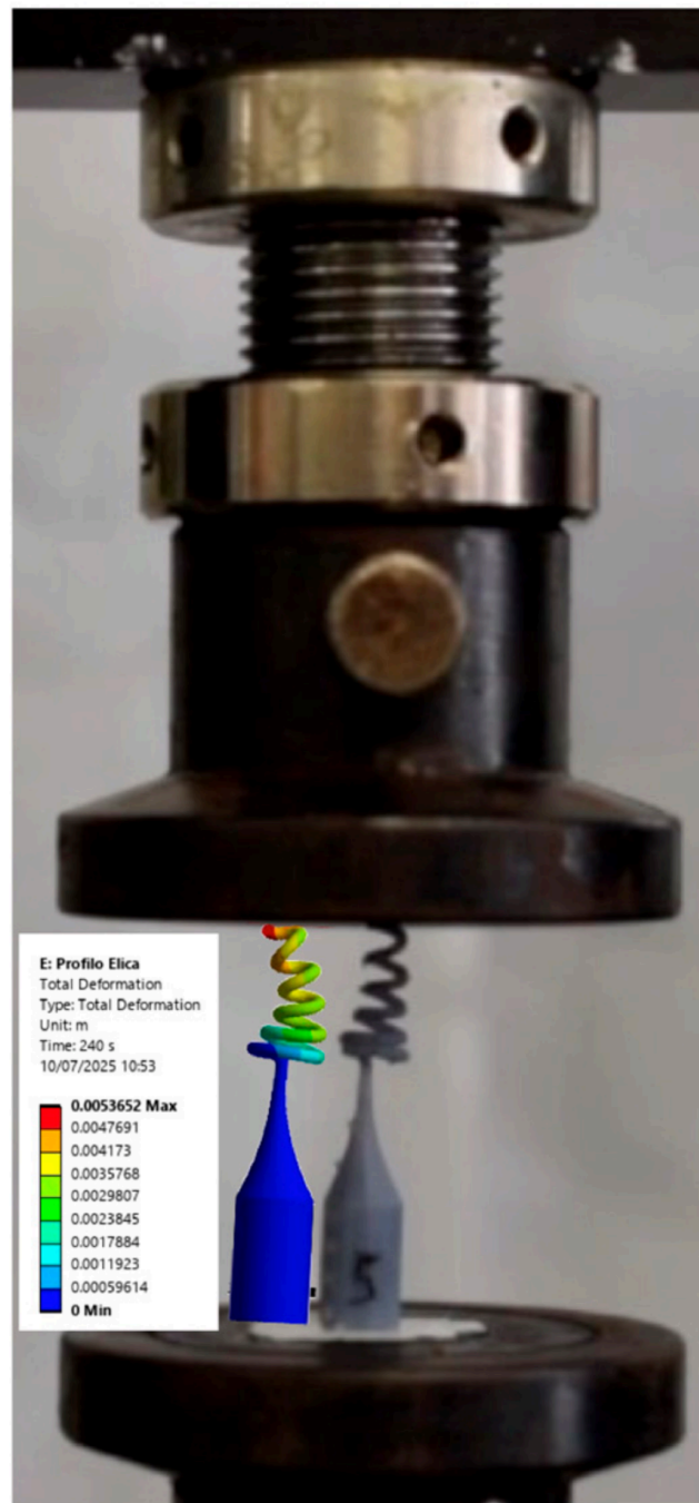
Figure 8. FE model vs. experimental swab deformations after 240 s of compressive testing.
