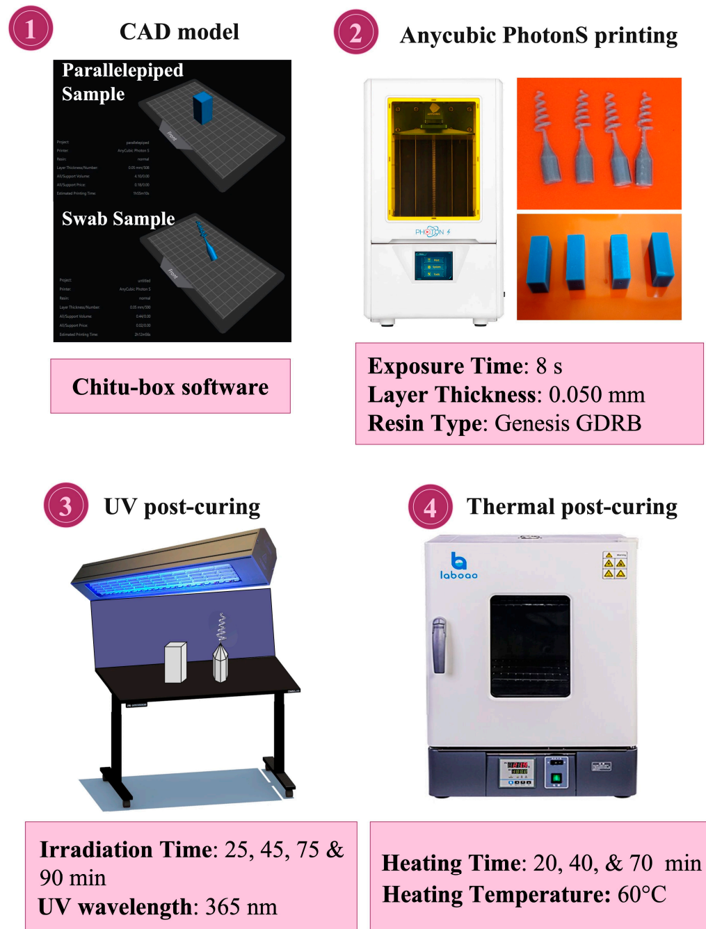
Figure 2. Schematic representation of the 3D printing process and the following post-curing treatments.
