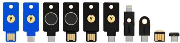
Fig. 1 Some examples of commercially available hardware authenticators produced by Yubico [16] working with FIDO2 Project's protocols and WebAuthn standards
