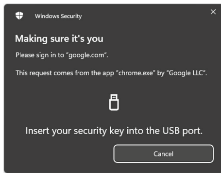
Fig. 25 Security window spawned by native Platform WebAuthn API on the victim's host OS (in this case Windows 11)
