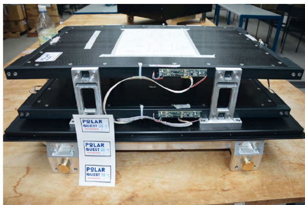
Fig. 2 One of the POLA-R detectors. Two planes of plastic scintillators, with four tiles each ( 30 \times 20 cm 2 ), are separated by a distance of 11 cm, and operated in coincidence as a telescope
