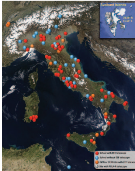
Fig. 1. – The map of the EEE network, that shows the location of the involved sites with different symbols: schools with MRPC telescopes, schools that joined the project without hosting a telescope, and a few sites where telescopes are installed inside CERN, INFN or University centres. The inset shows the POLA-R scintillator detectors installed at the Svalbard.
