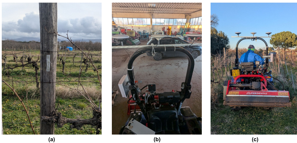
FIGURE 7. Details of the RFID-GNSS hardware setup. UHF RFID tags placed along the paths (a), the configuration of GNSS antennas on tractor's ROPS and RFID antenna on the left, (b) example of the operating conditions of the system in a vineyard (c).
