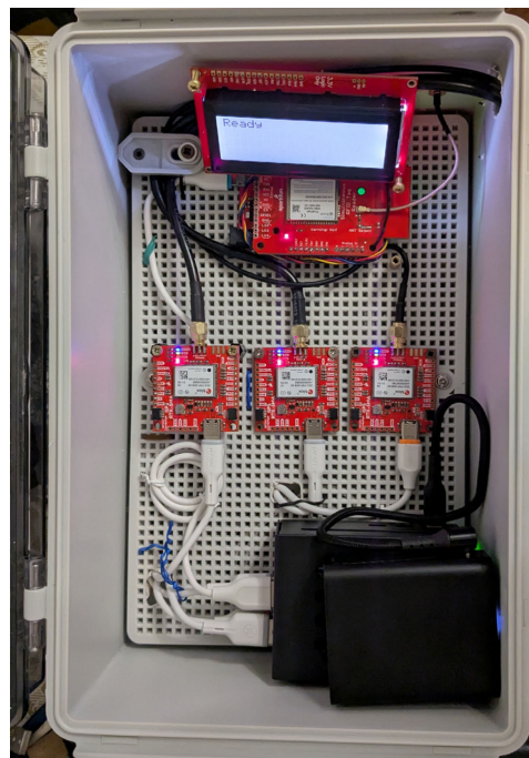
FIGURE 4. Hybrid RFID-GNSS circuit physical implementation.
