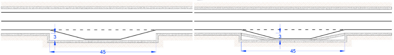
Fig. 3. (left) local widening of the tunnel cross-section in correspondence with lay-bys (with example measures taken from Italian standards). (right) solution representing the implementation of oblique vertical walls in presence of lay-bys.
