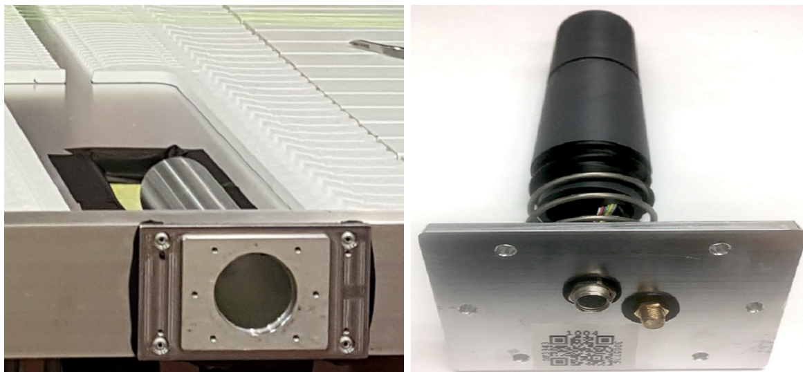
Figure 5. Left: aluminium tube housing the readout device. The tube separates the electronics from the inner detector components and is fixed with glue and rivets onto the frame beam. Right: the PVC tube containing the PMT unit. Visible are the spring to push the PMT to the end of the aluminium tube and the flange to close the aluminium tube.
