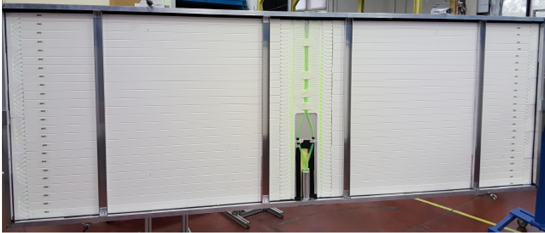
Figure 7. An open SSD where the scintillators have been secured with the tensioned aluminium bars. The polystyrene routers and the fibers are also visible.
