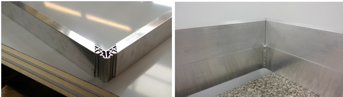
Figure 9. Left: technique to make SSD frame corners by gluing extruded aluminium profiles to corner connectors. Right: prototype frame corners made using the gluing and welding techniques.
