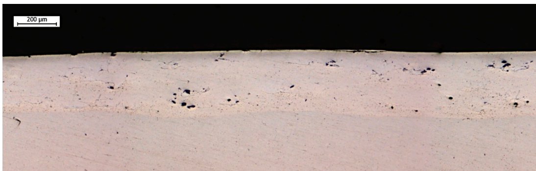
Figure 6. Cross-section (Plane XY) of ESD + UPT coating on AlSi10Mg substrate.
