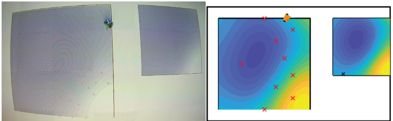
(B) The robot explores the domain using the SIEVE. The positions explored by the robot are depicted in red. After exploring 10 points, an estimation of the density function is computed. The contour line of the estimated function is shown in the left square of the image
