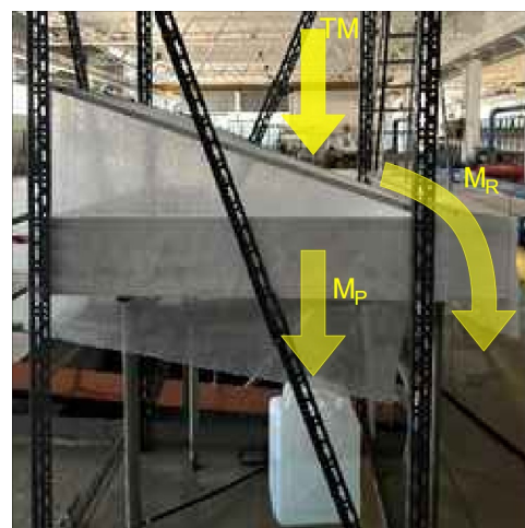
Figure 3. Containers below net ( TM stands for total water mass, M_P is the total pass-through water mass, M_R is the total runoff water mass).
