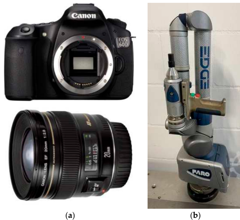
Figure 4. The (a) camera and lens and (b) Faro ScanArm2 used for the survey.
