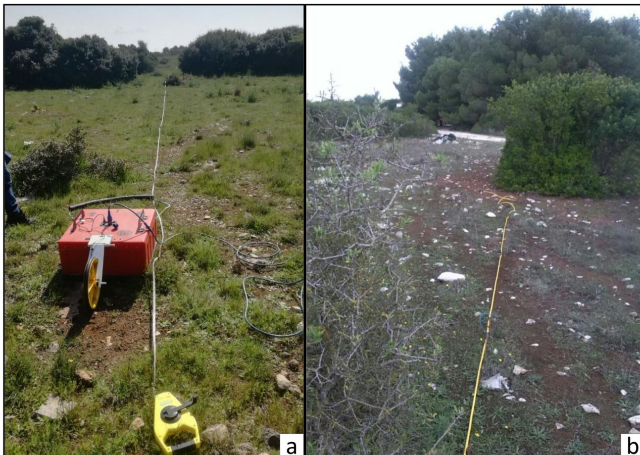
Figure 3. Images taken during the GPR (a) and ERT (b) surveys.
