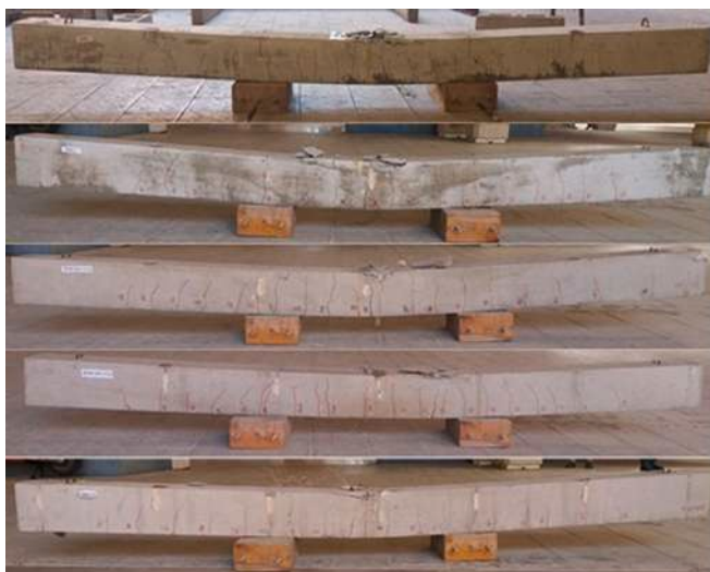
Fig. 7. Failure mechanism for LL Beams.
