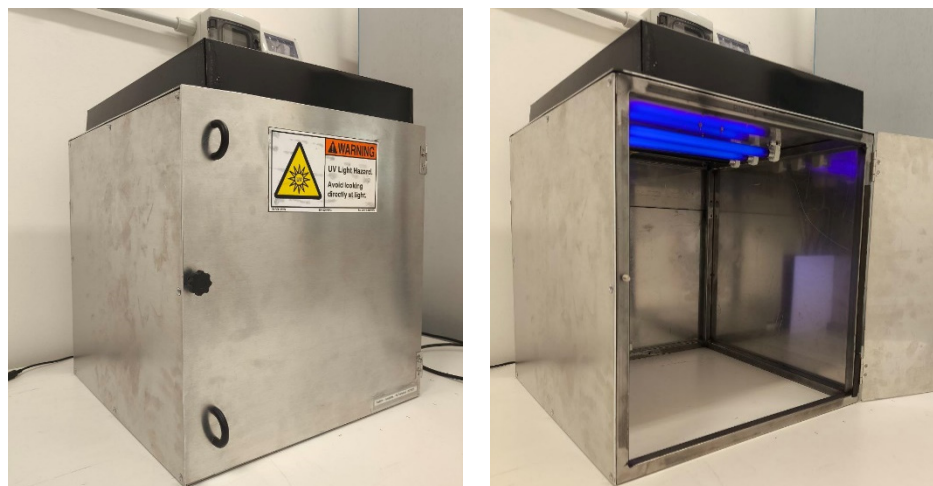
Figure 8. Pictures of the UV irradiator used for photocatalysis experiments.
