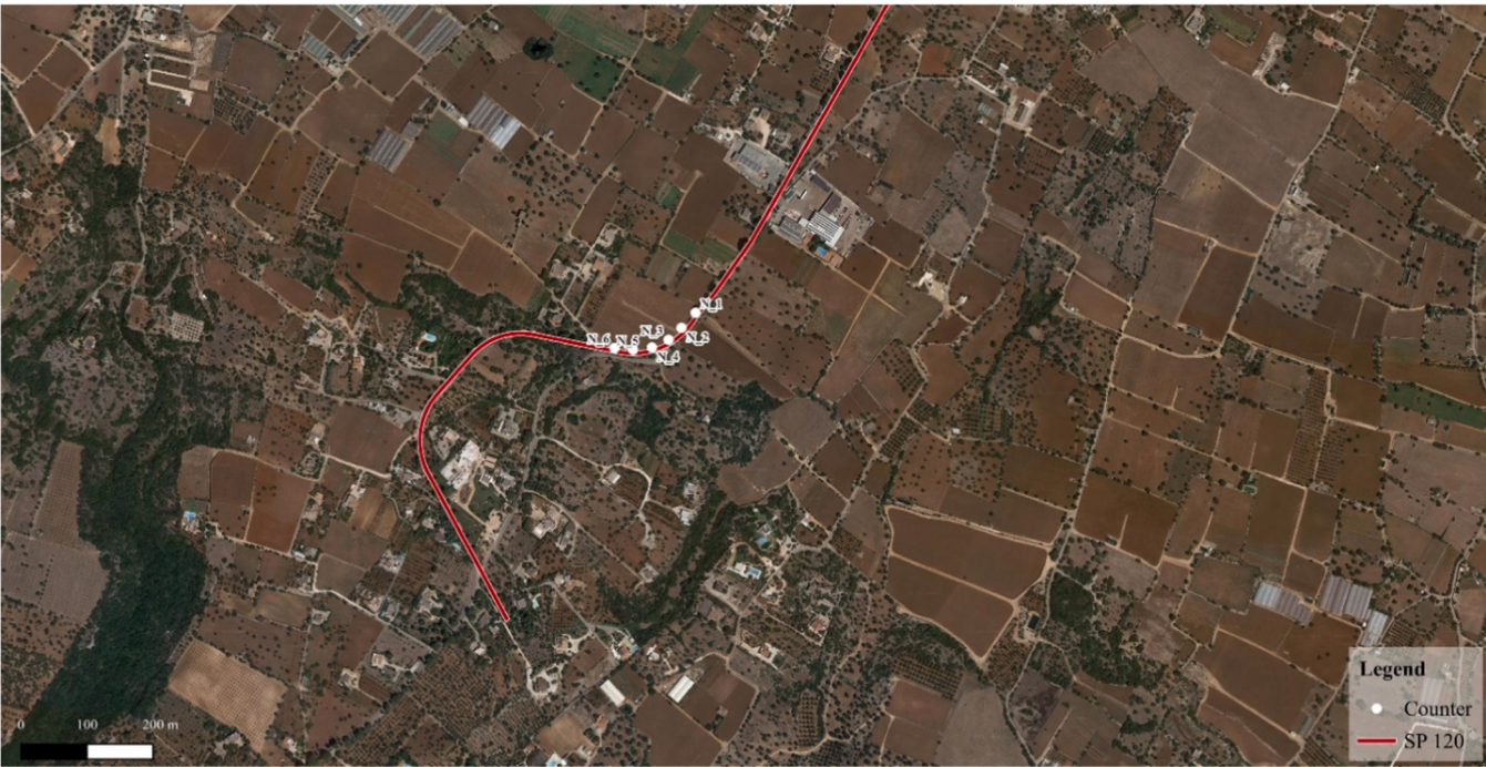
Fig. 3. Location of the 6 traffic counters (numbered from #1 to #6) on the selected section of the SP120. The spatial gap between two consecutive counters is equal to 30 m (colored figure). Image source: Google Satellite.
