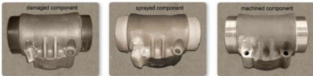
Fig. 34. Restoration process of a mechanically damaged flap transmission tee box housing of an aircraft via CSAM [133].
