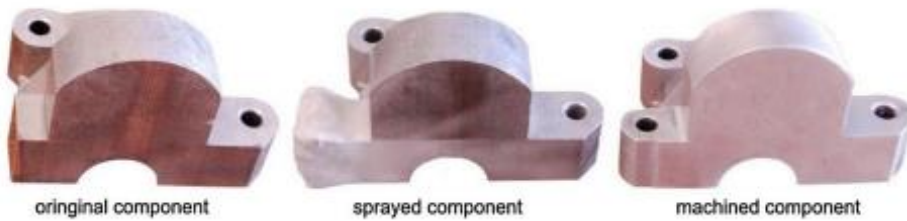
Fig. 26. Component with complex structure made by CSAM [71].
