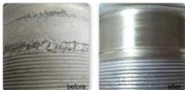
Fig. 33. Restored B737 nose wheel steering actuator barrel via CSAM [133].
