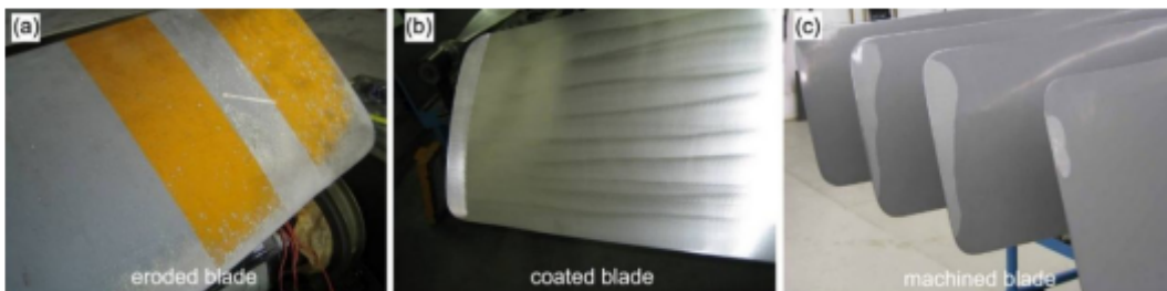
Fig. 39. Restoration process of aluminium alloy blades via CSAM [151].
