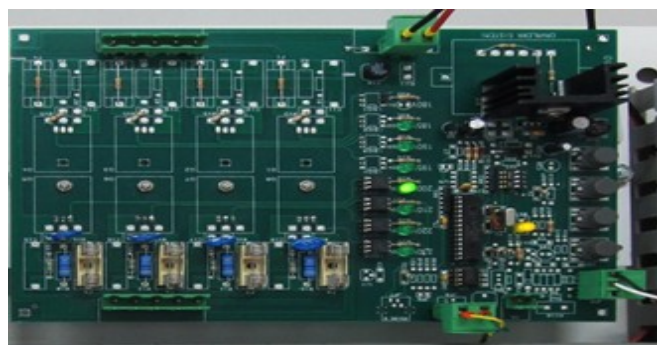
Figure 4a. C107 Master electronic board of PV plant with bi-axial solar tracker
